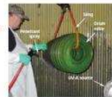
Figure 1. Surface of drum rotor is covered thoroughly and systematically during penetrant application. UV-A source is used to ensure all surfaces have been covered.
