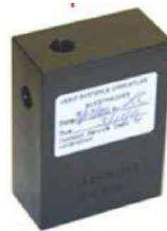
Measurement Verification Block With UV Target
